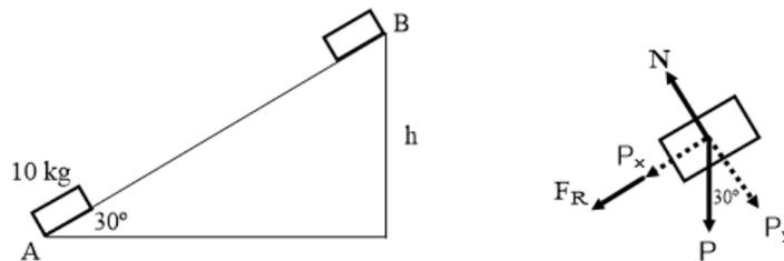
$$(i) \sin 30^\circ = \frac{h}{AB} \Rightarrow \overline{AB} = \frac{h}{\sin 30^\circ} = 2h ; F_R = \mu \cdot N = \mu \cdot P \cdot \cos 30^\circ = 0,1 \cdot 10 \cdot 9,8 \cdot \cos 30^\circ = 8,49 \text{ N}$$
