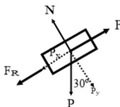
$$\left. \begin{array}{l} P_x = P \text{sen } 30^\circ = 100 \cdot 9'8 \cdot \text{sen } 30^\circ = 490 \text{ N} \\ P_y = P \text{cos } 30^\circ = 100 \cdot 9'8 \cdot \text{cos } 30^\circ = 848'7 \text{ N} \\ F_{\text{roz}} = \mu \cdot N = \mu \cdot P_y = 0'2 \cdot 848'7 = 169'74 \text{ N} \end{array} \right\} \Rightarrow F - F_{\text{roz}} - P_x = 0 \Rightarrow F = 169'74 + 490 = 659'74 \text{ N}$$
